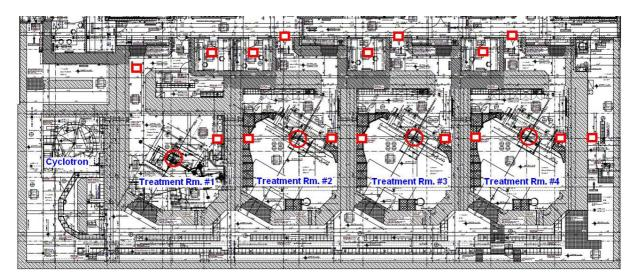
Figure A.1.1. Showing the treatment rooms of the WPE facility, which is based on an IBA Proteus 230 room temperature proton cyclotron, one fixed beam Treatment Room (#1) and three gantry Treatment Rooms (#2 - #4). The circles and rectangles indicate the radiation sources (proton impact points) used for radiation safety calculations and locations of neutron and gamma dose equivalent rate measurement respectively.
